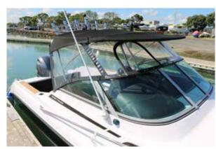
Model Haines Hunter SF635 Price as tested \$130,000 Priced from \$118,000 Type Cabin Boat Construction GRP LOA 6.76m Beam 2.34m Deadrise 21 deg Trailerable weight 1800kg Test Power 175hp Yamaha Fourstroke Power options Outboard HP Range 150hp-200hp Fuel Capacity 195L Trailer Tandem Axle Manufacturer Haines Hunter Ph 09 579 9661 www.haineshunter.co.nz
